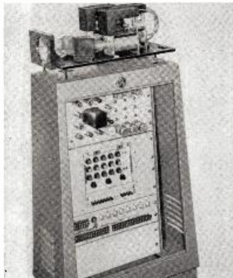
THIS IS General Precision Labs' recently-developed three-vidicon color film chain, model PA-520, which the firm says is especially compact and simple to operate. A field lens and filtering system for each channel are mounted on the camera head.
