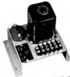
RI-108-6 AC POTENTIAL UNIT — used in the Rust System to remotely indicate AC line voltage or regulated filament line voltage (which is proportional to actual filament voltage). The unit is designed for operation on either 115 volts or 230 volts 50/60 cycles.
