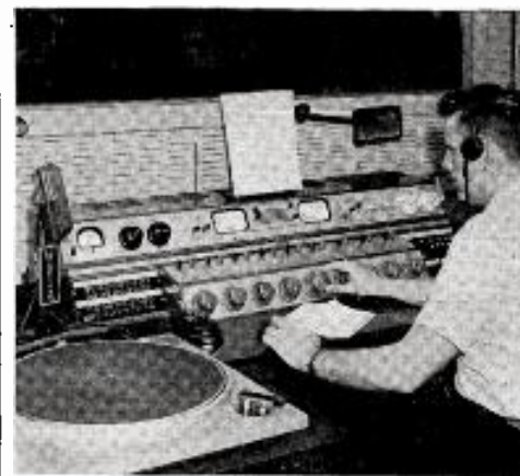
Altec 250 A speech input console controls WDIA program schedule. Completely self-contained, it provides all the necessary circuits for audio control.
