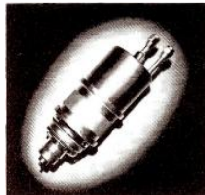
EIMAC'S 4W20,000A, with indirectly heated thoriated tungsten cathode, final amplifier in the Du Mont 25 KW VHF-TV transmitter, is the highest-power member of the famous Eimac radial-beam power tetrode family. The tetrodes feature high power gain and low driving power requirements.
