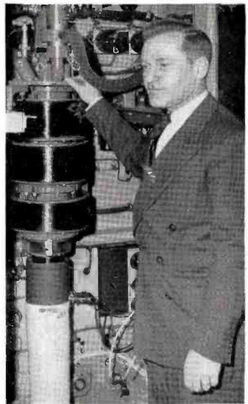
● Heart of Channel 61's powerful transmitter is the 15-kw G-E klystron tube at Chief Engineer Townsend's right. It airs WWLP's television signal over a wide radius. Clear pictures are further assured by the 320-foot transmitting tower based 640 feet high on Provin Mountain in the limits of the town of Agawam.
