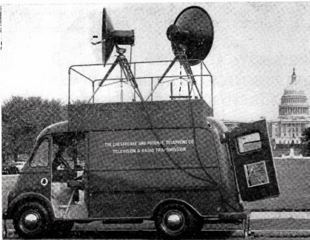
SET UP for operation, a Chesapeake & Potomac Telephone Co. mobile microwave relay unit is ready to pick up TV picture signals and relay
