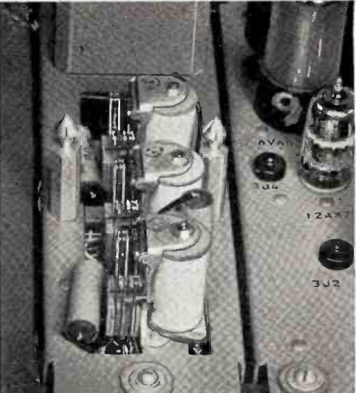
Improved, faster-operating speaker relays eliminate key clicks and audio feedback.
