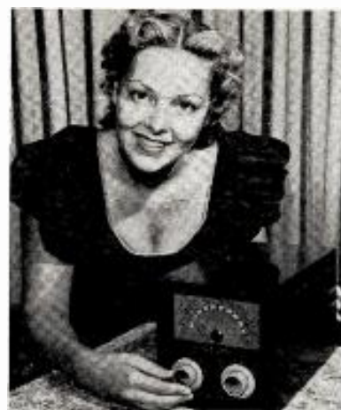
ATTRACTIVE Evelyn Miller of Syracuse demonstrates General Electric's new UHF translator which was shown to FCC officials, manufacturers and others June 29 in Bridgeport, Conn. [BROADCASTING • TELECASTING, July 2]. The unit, which GE says can be used with any TV set, provides continuous tuning, covering the UHF band from 475 to 890 mc.
