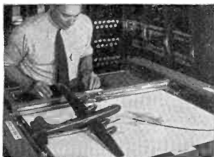
Here you see models of a guided missile and a bomber about to meet on the plotting board of RCA's computer.
