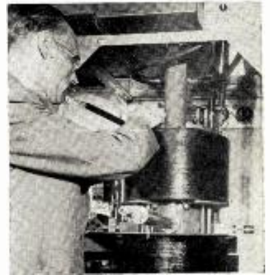
H. M. CROSBY, General Electric engineer, adjusts a new UHF velocity-modulated tube around which GE has built a 5 kw UHF television transmitter at Electronics Park, Syracuse. Transmitter will operate in the 500 mc region. GE announced the development at the IRE meeting.
