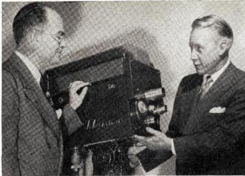
This camera, CBS says, will be used to operate its color system as approved by FCC. Pointing out highlights to Mr. Terry (l) is Frank Stanton, CBS president. Camera is standard black-and-white modified for CBS standards by RCA.
