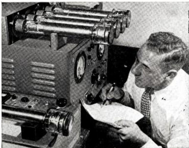
Here, in a testing battery at RCA Tube Plant in Lancaster, Pa., RCA image orthicon pick-up tubes get the final seal of approval from an engineer.
