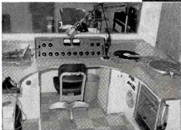
KFJI's new Collins 212A speech input console
