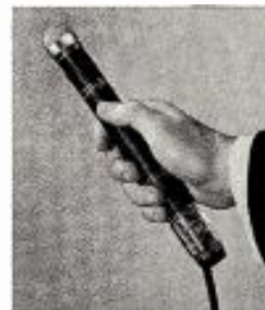
Shows TV 655 in the hand with swivel removed. Note how convenient it is to handle for announcing or interviewing.
