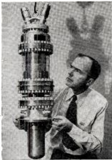
RCA'S NEW "super-power beam triode" which is capable of 500 kw output is examined by Dr. L. P. Garner, head of the Advance Development Lab. of the RCA Lancaster, Pa., tube plant, where the tube was developed. Weighing only 135 lb and measuring 38 3/4 in., the tube is now commercially available.
