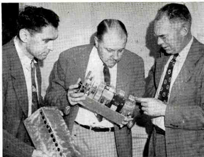
AN 11-TUBE automobile radio that will tune the entire FM band has been made for station cars of WPJB, FM station of the Providence Journal . The new set, less than six inches square and a foot long, is examined by H. William Koster (center), WPJB manager. With Mr. Koster are George Sharpe (r), station engineer, and Charles Snell, representing Barber & Howard, a Westerly, R. I., electronics research firm which developed the set. Mr. Snell holds the aluminum case in which the receiver is mounted.
