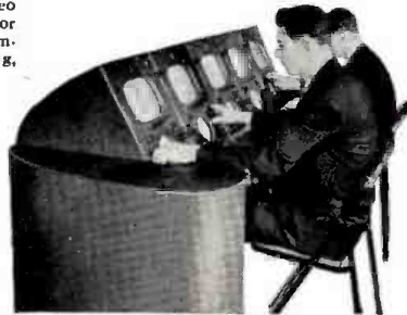
VIDEO CONSOLE —composed of studio and film camera controls, a master monitor, and switching, lap-dissolve, and fading facilities for selecting the camera pick-up desired. "Building-block" design assures a compact, unified appearance . . . permits adding extra units at any time.
