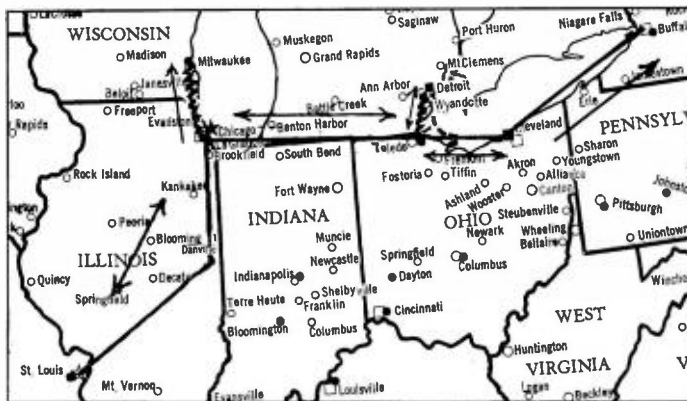
Heavy inked lines represent coaxial cable and wavy lines relay towers. Two-way arrows indicate that stations can both receive and transmit insofar as cable or tower facilities permit. One-way arrow indicates that station located in place pointed to can only receive.
