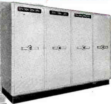
FEDERAL'S FM 10 KW Transmitter , officially approved by the FCC, has the exclusive "Frequentomatic" FM Modulator. It reduces distortion and noise well below RMA specifications, and stabilizes mean carrier frequency within 0.001 per cent of assigned value. This transmitter combines outstanding fidelity with economy, accessibility and highly dependable performance.
