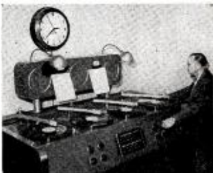
Recorded musical programs originating at this specially-designed transcription machine at WJR Detroit are safe-guarded against surface noise and bass rumble by the *Dynamic Noise Suppressor in the Control Room. Results: vastly improved quality in all WJR recorded musical programs.
