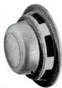
755A 8" direct radiator, 8 watts capacity. Response 70 to 13,000 cps.
