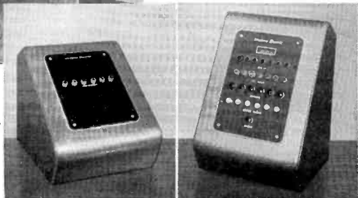
● Below—Flash Booth Indicator Panel (at left) and Control Signal Indicator Panel (at right).
