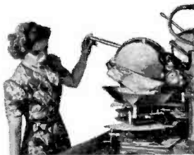
On the "production" front — a Federal Telephone and Radio technician "aims" her modern crystal-cutting saw.
