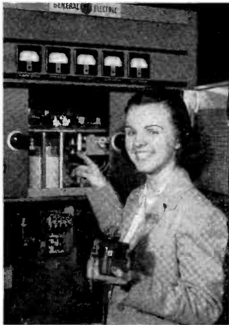
THIS YOUNG LADY is holding a tube and radiator specially designed for FM and television by General Electric engineers. She is pointing at another installed in the 3,000-watt FM transmitter, which requires two of these tubes, each capable of an 1,800-watt output for FM service and cooled by air blown through its copper radiator.
