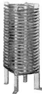
ES-675768 RF Isolation Coil for bypassing phase monitor sampling lines around tower insulator.
