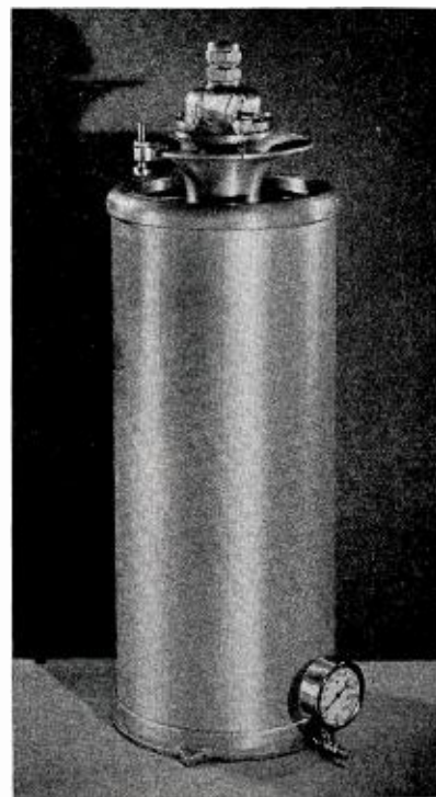
Lapp variable condenser Y150V15 100 amp., 15KV (carrier RMS, 100% modulation) Capacitance 600-1500 mmf. External dimensions: Height 34", diameter, 11".
