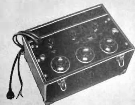
PRESTO PREAMPLIFIER AND MIXER — For use with Presto Recording amplifier. Consists of three channel mixer, two stage amplifier and power cable in carrying case. Also available for relay rack mounting.
