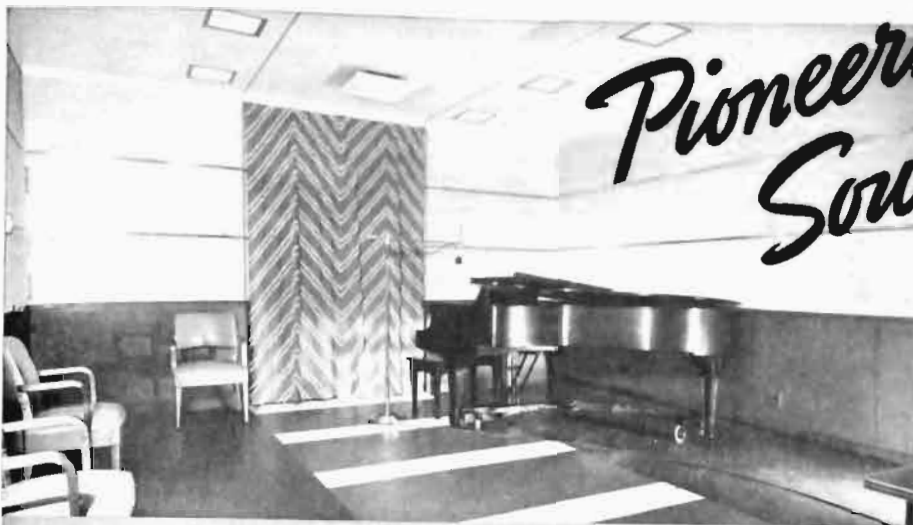
One of the new WWJ studios treated on walls and ceilings with J-M Sound-Control Materials and isolated from the rest of the structure by the J-M system of sound isolation. Note the adaptability of the material to the modern decorative style.
