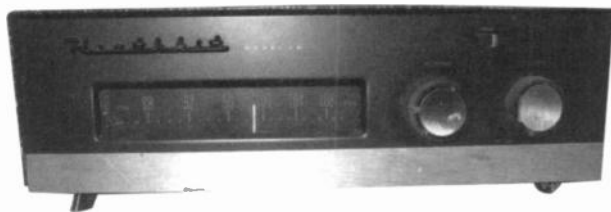
Heathkit Model FM4 FM Tuner – Early FM tuner from Heathkit. There are 5 tubes. Manufactured about 1960. Steve Goh, Sioux Falls, SD.
