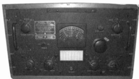
US Navy Model CRV-46148 Communications Receiver – Made by RCA for the US Navy. Covers 4.0 Mhz to 27 Mhz. Robert Vogel, Deerfield, FL.
