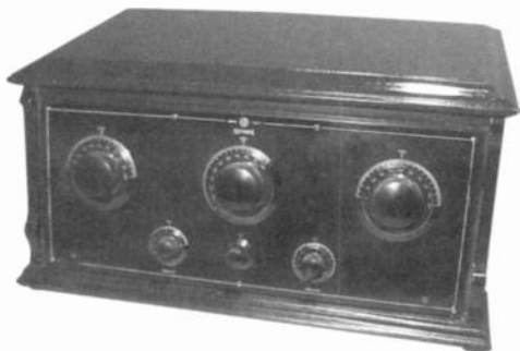
FADA (Frank Angelo D'Andrea), Model 175 - A five-tube receiver of 1925. FADA was one of the first radio manufacturers to incorporate the Hazeltine Neutrodyne circuit in their radios. FADA lasted well into the 1950's with radio and Television products. Dave Crocker, Mashpee, MA.
