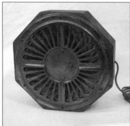
Utah drum speaker back view. The top and bottom screws in the center hold the balanced armature mechanism to the grille. The other screw to the center right is the leaf centering adjustment.
