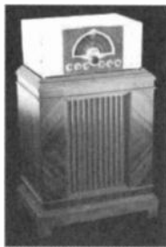
The 1936 McMurdo Silver Masterpiece V ranked Seventh. It was purchased, electronically restored and aligned in 2009. It is completely original with the exception of the cover being re-chromed, it has the re-coated 18" Jensen speaker and Clifton cabinet with the back.
