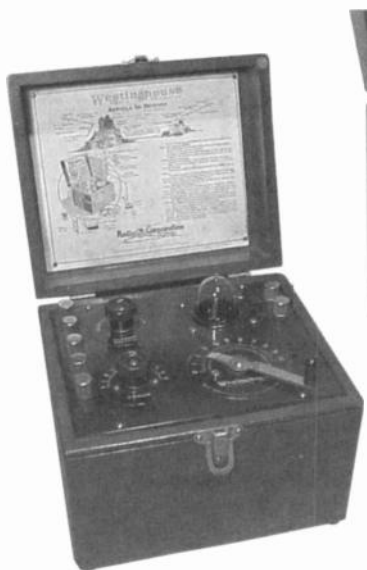
Westinghouse Aeriola Sr. 1-tube receiver of 1921. Although the "Westinghouse" name is on the set, it was sold through the RCA marketing division. The first Aeriola had a wooden panel with silvered dials. This later version has an all-Bakelite panel. Dave Crocker - Mashpee, MA
