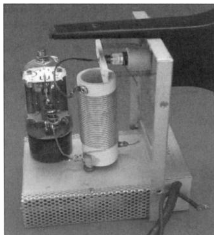
The Ionovac speaker seen in operation with the bluish purple glow of the plasma.
