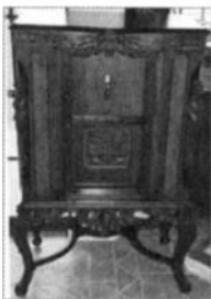
The 1952 Zenith 12 Deluxe ranked Sixth. It was completely disassembled, all metal parts re-chromed and re-assembled and aligned in 2010 and placed in a 1980s Palco cabinet, it has the original Bush and uses a Jensen A12 speaker.
