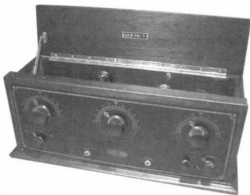
Day-Fan Model OEM-7 four-tube receiver of 1924. It has a gold, silk-screened Bakelite panel. Dave Crocker, Mashpee, MA
