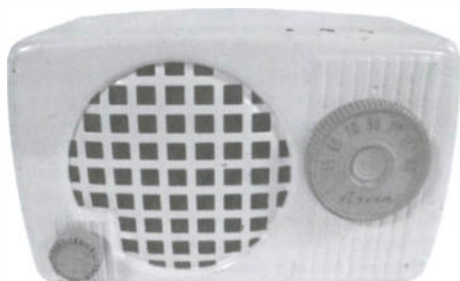
Arvin model 440-T radio – This midget radio was made in 1950. It covered the AM band and had four tubes. James Simeone, Billings, MT
