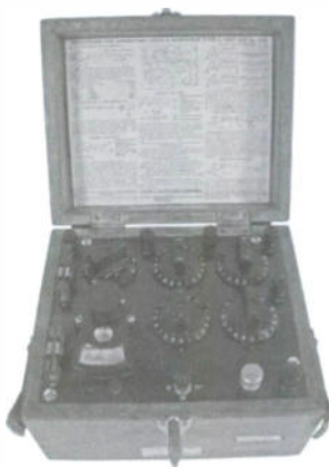
Leeds & Northrup model 5300 Type S test set – This piece of test equipment was known as a Wheatstone Bridge. It is a precision ohm meter used to measure various resistances. Cabinet is made of wood. Curtis Beardsley, Taos, NM
