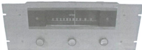
Craftsmen model 900 – This is an FM Tuner from the 1950s. Craftsmen was known for their chrome chassis. This version had a rack mounted front panel. Andrew Dietrig, Newhall, CA
