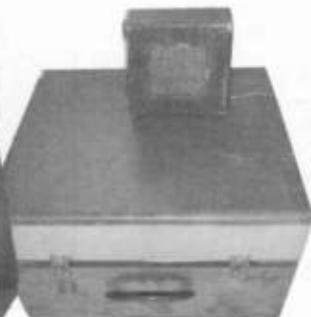
**Motorola SH18GL Portable Phonograph** – This “portable” phonograph weighs about 45 pounds. Has six tubes and two detachable speakers with 10 feet of wire. Made in 1959 with a four-speed record changer. *Ari Hourani - Bangor, ME.*
