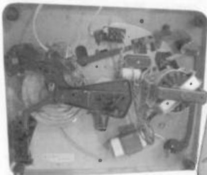
**Benjamin Miracord Elac 10H turntable** – German made turntable from the early 1960s. Played at speeds 16, 33, 45, 78 RPM and 7", 10", and 12" records. Came with spindle to stack records. *Norman Hughes - San Francisco, CA.*
