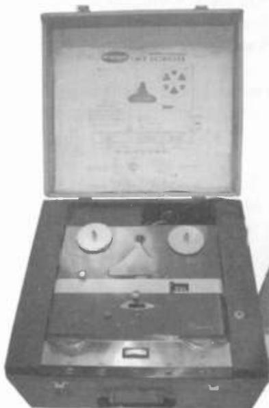
**Penron HF-400 Reel-To-Reel Tape Deck** – Manufactured in 1956. This mono deck was called the “Emperor” and has two speakers in the cabinet and one external speaker referred to as a tweeter. There are seven tubes. *Sam Goetzmann - Memphis, TN.*
