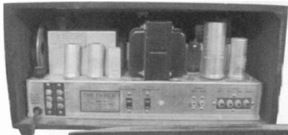
**Fisher model 90-T** – This is an AM/FM mono tuner pre-amplifier manufactured approximately 1958. It features a tuning eye and inputs for phono, tape, aux 1, and aux 2. *Arthur Morris, Englisht:cwn - NJ.*
