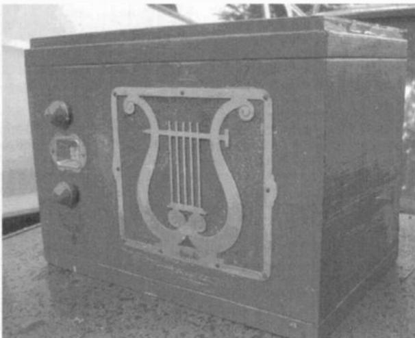
reception and sound quality is very good, probably the best of Smart Set series of radios, mainly because of the two IF stages and separated audio and AVC detection circuits. A 10-inch-long external antenna works very well, and I was able to pick up more than 15 stations on the AM band and every signal was clean, crisp and very clear. There was no hum, static or buzzing.
