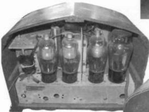
**Emerson model 250-AW** – manufactured in 1933. This is a five tube radio that covered AM and short wave. It has two knobs in front and the band switch in the rear. *Jerry Fulcrum - Sioux Falls, SD.*
