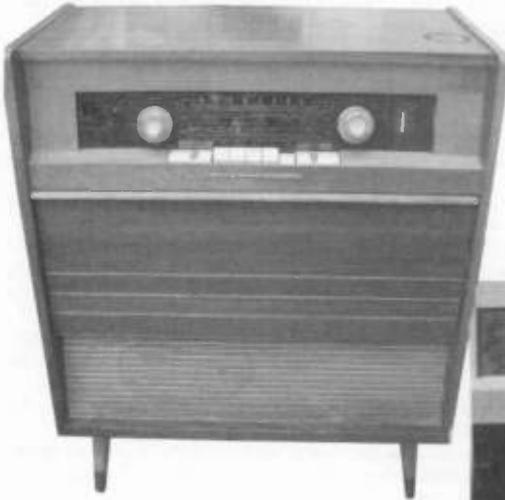
**Grundig Majestic model M1PX** – manufactured in Germany in 1958. This six tube mono radio/phonograph console covered the AM, FM, and shortwave bands from 6 mc to 16mc. The record changer is marked Grundig and came with the 45 RPM record spindle. *Roger Smith - Lawrence, KS.*
