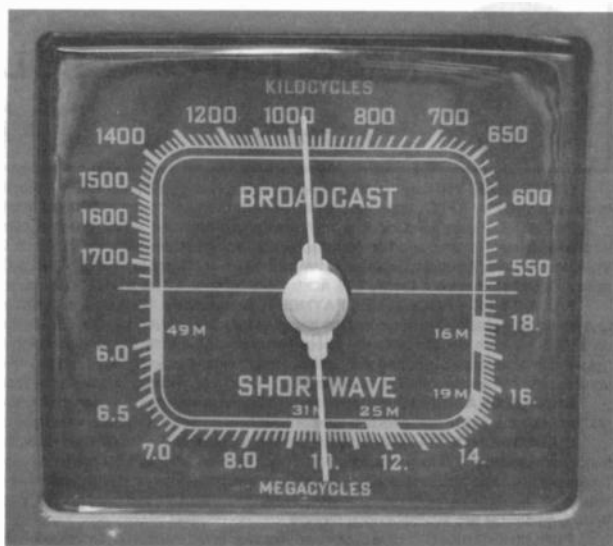
Figure 16. The new plastic dial cover mounted in the Templeone. Compare with the cracked dial cover shown in Figure 1.
