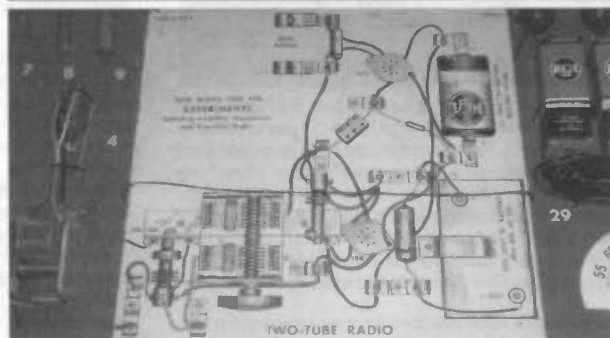
Geoffrey Bourne entered this Educational Hobby Kit in the equipment contest. With the Electronics No. 1 kit, you could build a two-tube radio receiver.
