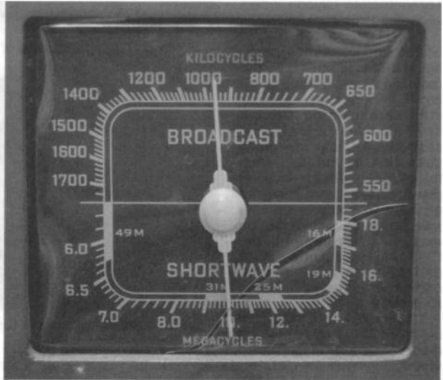
Figure 1. The cracked and deformed dial on my Templetone radio.
