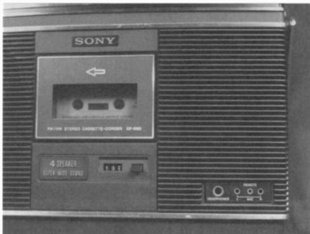
Figure 2. A close-up of the cassette drive.
