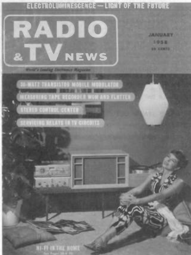
Figure 1. The Radio & TV News cover for January 1958 shows a "nicely styled, yet compact high-fidelity system." The speaker is a University Ultra-Linear S-10L 2-way speaker system with 12-inch woofer. The electronics are an H.H. Scott Model 99-D, 22-watt amplifier, and an H.H. Scott Model 330-C tuner with independent AM and FM sections. The turntable is a Rek-O-Kut B-12H.
