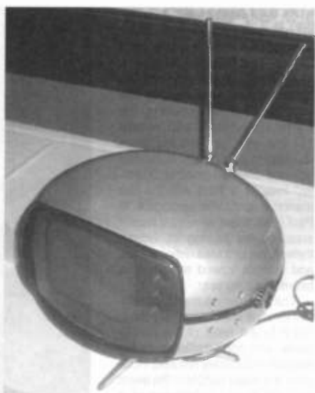
This 1971 Panasonic Model TR-005 "Orbitel" television set was entered in the contest by Jayne Kaiser. This 5" portable set included 22 individual transistors! The set reflected the fascination with the post-moon landing space travel.
