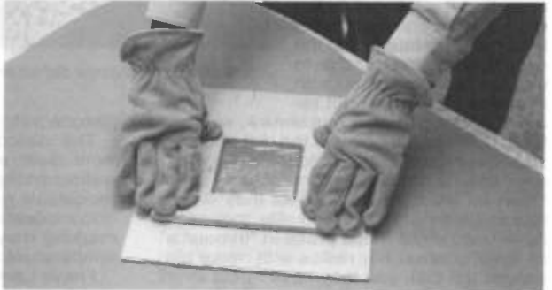
Figure 12. Press on the outer mold to form the new dial cover.
