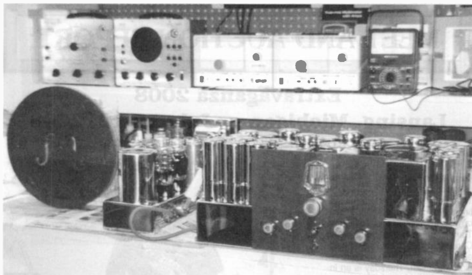
Figure 6. The completely restored Allwave 23 on the workbench for testing. Left to right, the speaker with an optional diffuser, the power amplifier/power supply, and the main chassis.
