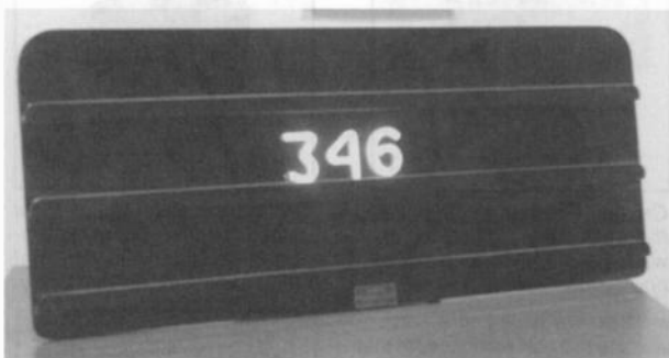
Figure 1. This view of the NeoNEON shows its black Plexiglas front panel and the three shelves with some numbers on the center shelf. Note the nameplate at the bottom of the panel.
