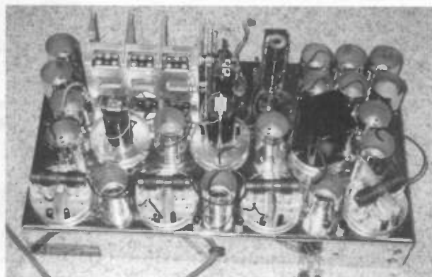
Figure 3. A top view of the upper chassis with tube and coil shields removed..
