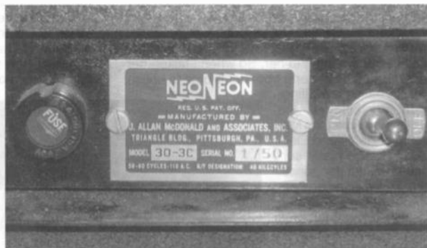
Figure 5. The transmitter has its own nameplate located between the fuse and On/Off toggle switch.
