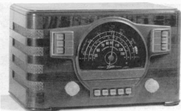
A 1941 Zenith table radio, Model 7-S-529. This 7-tube radio had seven tubes and covered the standard broadcast, shortwave, police and amateur bands.
