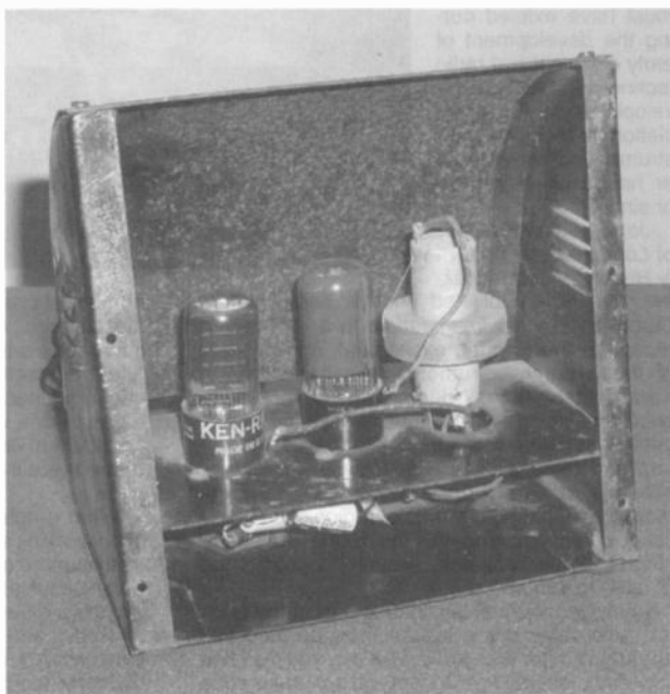
Figure 6. Shown are the two Type 50L6GT tubes and the 40 kHz oscillator coil.
