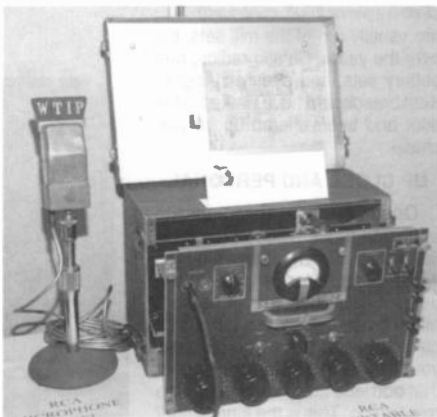
An interesting contest entry was this combination early RCA portable mixer and 74-B microphone.
