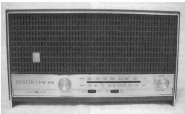
Figure 4. A Zenith Model A411, date coded September 1969, which has the heavy PC board riveted into a steel chassis.
