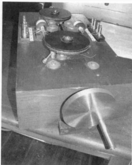
Figure 7. Another Marconi invention used in the early days of wireless — a magnetic detector.
