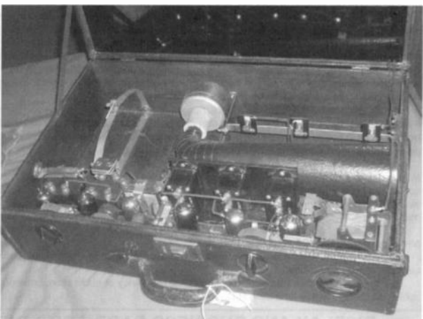
Rare is the word to describe this 1924 Zenith portable Model ZEV which brought a $7,500 bid. The lower photo shows an interior view of this set. Note the unusual horn and driver configuration.
