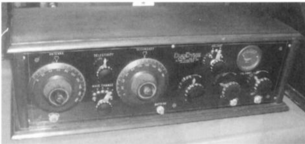
Look at all those knobs... and a meter, too! This Globe Electric DuoDyne 5-tube set sold for $280 in 1924. Without tubes, it sold here for $250. On the right is a close-up of the engraving on the panel.
