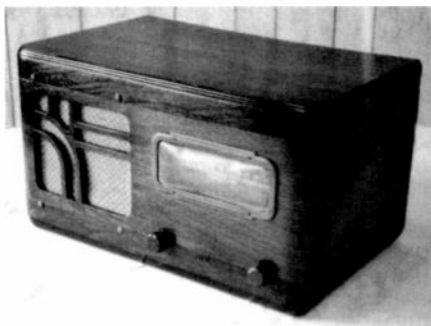
Figure 1. A Truetone Model D935 battery-operated "farm set." This 4-tube set is a 1940 model.
