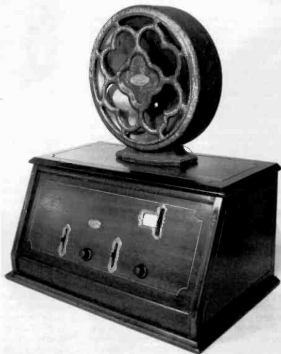
Figure 1. The Crosley Model 5-50 incorporated one-knob tuning. The single-tuning control is on the upper right of the slant-front panel. The thumbwheel is rotated up or down to tune in stations.
