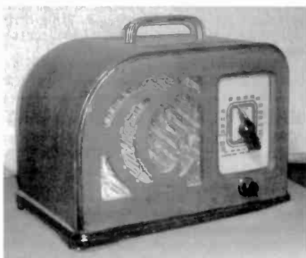
Figure 3. The third possible speaker location at the front of the cabinet was the final choice.
