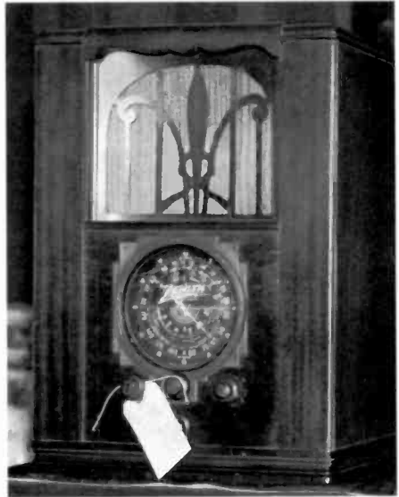
One of two Zenith tombstones housed in identical cabinets. The Model 6S27, an AC-operated radio, sold for $325. The Model 6V27, a wet cell-operated farm set, sold for $250.
