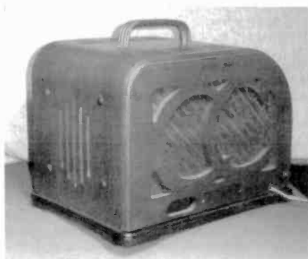
Figure 2. This rear view of the intercom shows two of the three possible mounting positions for the speaker.
