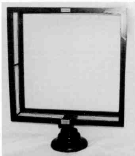
This original loop antenna with a square format was called the "Portaloop." It was manufactured by Eagle Radio Company of Newark, New Jersey, maker of a complete line of radio receivers.
