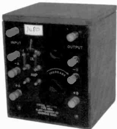
CLAPP-EASTHAM TYPE HRA – This 1-stage amplifier was made for use with the Clapp-Eastham Type HRD detector panel set. It was manufactured in 1921 by the Clapp-Eastham Company of Cambridge, Mass. ( Wally Worth – Wollaston, MA )
