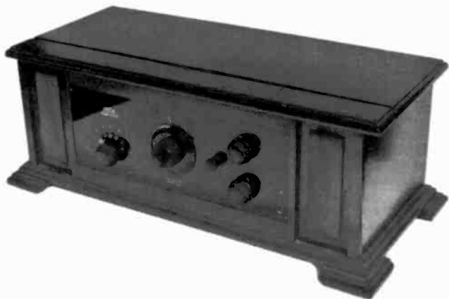
EDISON BABY GRAND – A seldom seen set, this early battery receiver, manufactured by the Edison Corp. in Chicago, Ill., uses four Type UV-199 tubes. (Ray Chase – Plainfield, NJ)
