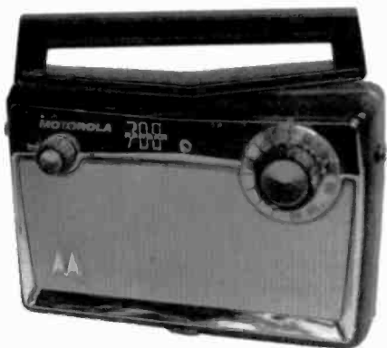
MOTOROLA RANGER 700 – This AC/DC/battery-operated portable has a rotatable loop antenna built into the handle. It features lots of chrome trim. ( Ray Chase – Plainfield, NJ )
