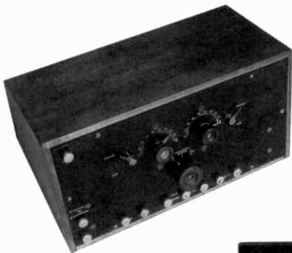
WIRELESS SPECIALTY APPARATUS IP-503 – This long-wave unit is used with the IP-500 or IP-501 receivers to extend their tuning range for long-wave reception. (Dave Crocker – Mashpee, MA)
