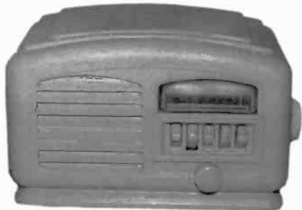
AIRLINE MODEL 04BR514 – This stylized Deco radio, housed in a painted Bakelite cabinet, was sold in 1940 by the Montgomery Ward Company of Chicago, Illinois. The chassis has 5 tubes and 5 push buttons. ( Clark Trissell – Lincoln, NB )
