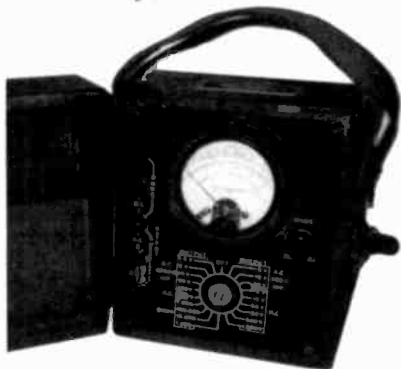
SIGNAL CORPS I-166 VOLT-OHMETER – This volt-ohmmeter was manufactured in 1944. It requires a 4 ½-volt battery for operation. It is rated at 1,000 ohms per volts, DC. (Louis L. D'Antuono – Brooklyn, NY)
