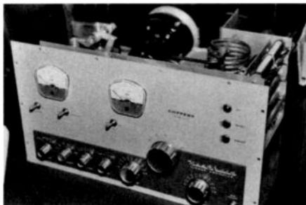
This Heathkit Model KL-1 "Chippawa" HF linear amplifier with power supply, but less cabinet, sold for $400.
