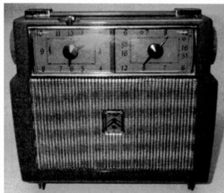
Figure 1. The "Missing Link Portable," a Motorola Model 53LC3. The set is unusual because of its tube complement and mechanical clock.
