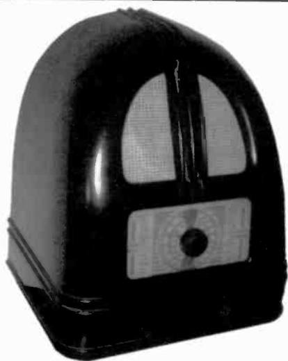
PHILCO MODEL 444 – This Bakelite cathedral radio was manufactured in the United Kingdom in 1936. Called "The Peoples Set," it is a 4-tube superhet that tunes medium and long wave bands. It was a low-cost set selling for $25 (U.S.). ( Jim Taylor – Bournemouth, England )
