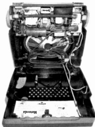
Figure 4. An interior view of the radio with what first appeared to be a damaged speaker.
