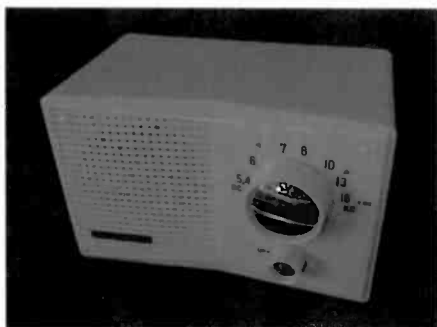
Figure 1. This radio branded the Sorrento shares the same chassis as other brands. Note the Civil Defense markings on the tuning scale.
