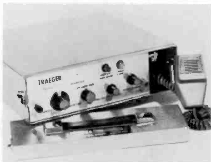
Figure 11. By the 1970s, the Adelaide workshop was turning out a different product like this single sideband set.
