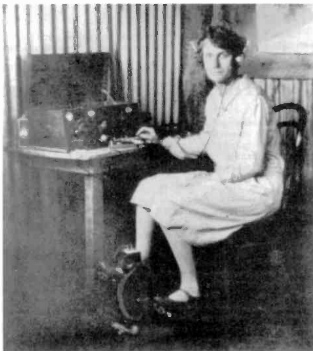
Figure 4. Once telephony had become feasible, the pedal outfit provided complete communication for the isolated homestead. Here, Mrs. Gertrude Rothery of Augustus Downs, operates the first pedal radio on June 19, 1929.
