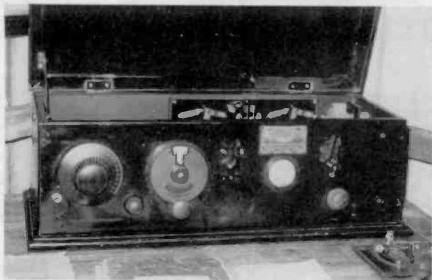
Figure 5. Transceiver Set #1, ca. 1930, reconditioned and encased in a metal cabinet. Note the telegraph key at right.
