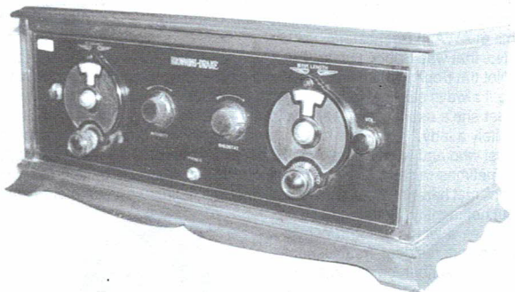
Figure 1. The Browning-Drake Model 5R with variable ratio vernier dials at either end of the cabinet.
