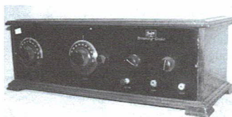
Figure 2. A Browning-Drake 4-tube set with both dials at the left-hand side of the panel. Note the Browning-Drake engraving with the "Baird Built" logo just above.
