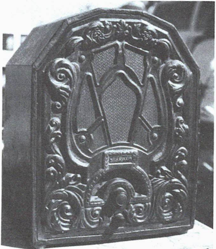
A beautiful example of a working Hartco 4-tube cathedral with a leatherette-covered cardboard cabinet, seen outside in the lot at Jerry Finamore's table.
