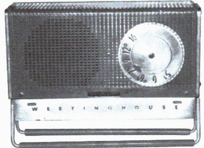
WESTINGHOUSE MODEL H-493-P4 — This Art Deco portable uses subminiature tubes—Types 1V6, 1AH4, 1AJ5 and 1AG4. Measurements are 6-inches long, 3 3 / 4 -inches high not including the handle, and 1 3 / 4 -inches deep. ( Francis Buren — Postville, IA )
