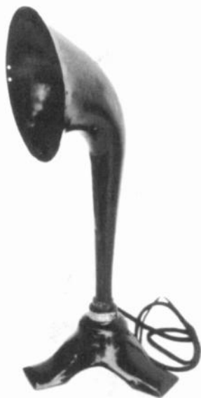
WESTERN ELECTRIC MODEL 517W – This rather crudely made, black painted brass horn speaker has a bell diameter of 5\frac{1}{2} " , with an overall height of 16\frac{1}{4} ". Note the two small holes on both sides of the bell mouth. The decal at the top of the base identifies the horn. I'm seeking more information, which can be forwarded to A.R.C. ( Ed Bell – Raleigh, NC )
