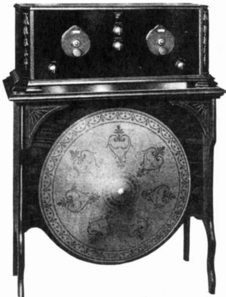
Figure 1. A Samson Electric Model T/C and cone loudspeaker installed in a console cabinet.
