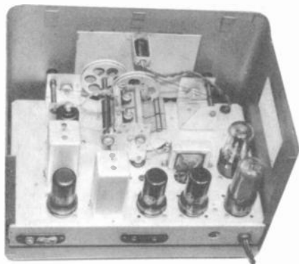
Figure 2. A view of the EC-1, minus cabinet top and speaker, reveals the simple layout of this inexpensive set.
