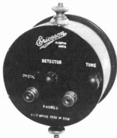
ERICSSON CRYSTAL SET, BRITISH – Made by the L.M. Ericsson Mfg. Co., Ltd., this 1924 circular Bakelite crystal set is only 3" in diameter. Note the post office registration number at the bottom. ( Jim Taylor – Winton-Bournemouth, England )
