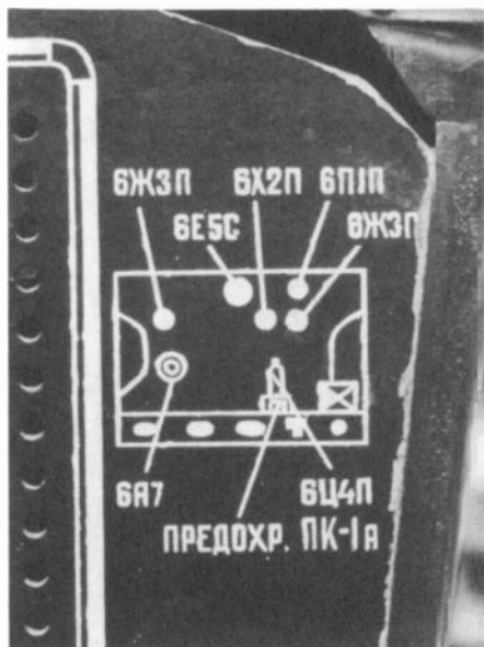
Figure 3. A diagram of the location of the Red Star 54's tubes.
