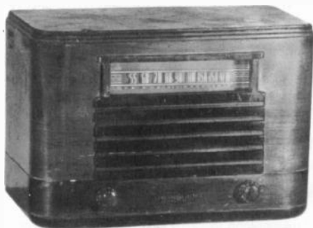
GENERAL ELECTRIC MODEL LCP-609 – This 1941 table radio has a 6-tube "Golden Tone" superhet chassis. It also features the famous GE Beam-A-Scope aerial. The cabinet is of walnut veneer with toning lacquer for contrast. ( Robert Bailey – Jacksonville, FL )
