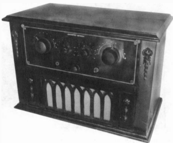
BRANSTON MODEL R47 HETROLA V – Made in Buffalo, N. Y., in 1925, by Chas. A. Branston, Ltd., this radio is a 5-tube TRF with integral horn speaker under the chassis. Branston had a Toronto office and advertised prominently in Canadian radio magazines. The company also made "medical" apparatus described in a 1923 radio ad as: "The famous Branston Violet Ray High Frequency Generators." ( Bob Murray – Winnipeg, MB, Canada )
