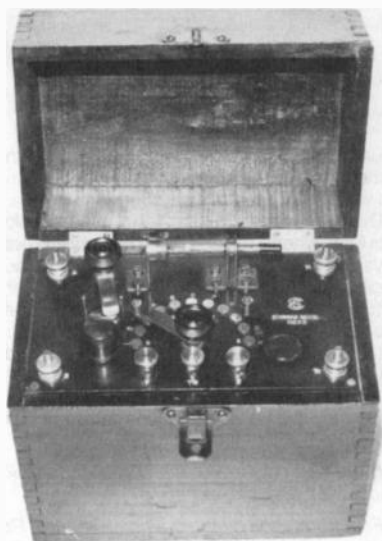
Figure 1. The Ediswan 1923B crystal set was purportedly being turned out of the Edison Swan factory at the rate of one every six minutes.
