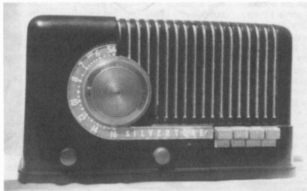
Figure 1. The Commentator Model 7004, a 5-tube superheterodyne with a built-in loop antenna in a surround plastic cabinet.
