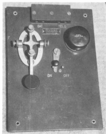
Figure 1. A Century code practice set built to train wireless telegraphy operators.
