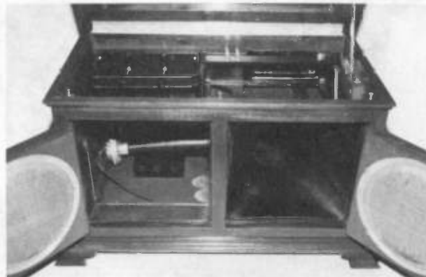
Figure 5. A view of the speaker assembly showing the driver and neck of the horn in the left compartment, with the horn taking up the right compartment.
