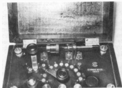
Figure 2. Close-up of the protective crystal cap in place on the 1923B. When not in use, the cap is screwed on the brass dome at the left of the tuning switch.
