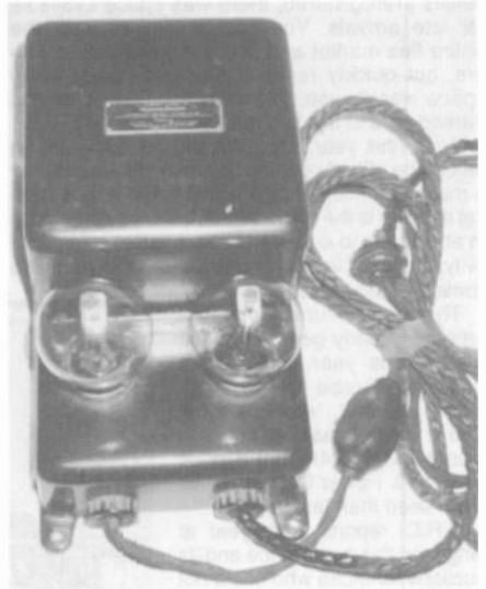
WESTERN ELECTRIC MODEL 2A – This power supply was used with the Western Electric Model 7A amplifier. Note the two Type 217A Western Electric "tennis ball" tubes. ( Ed Bell – Raleigh, NC )
