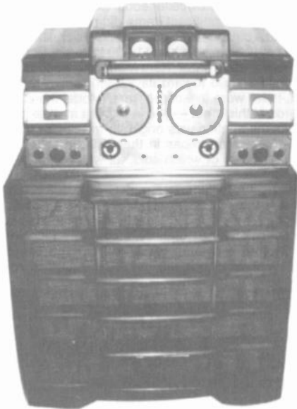
HALLCRAFTERS MODEL DD-1 – This late 1930s, single control, Dual-Diversity receiver has two complete RF, IF and second detector stages with a common local oscillator and audio stage. The radio selects the strongest signal to reduce shortwave fading. The power supply and audio amplifier are contained in a separate chassis. The set has 26 tubes and 3 "S" meters. ( Joel Levine – Greenlawn, NY )
