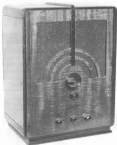
Figure 4. A Philco Model 60MB tombstone. The set is being restored because of the incorrect grille cloth and lack of vertical veneer strips on the front sides. (Photo courtesy of Ron Ramirez.)
