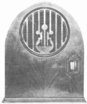
ECHOPHONE MODEL S-3 – This 1930 TRF cathedral radio uses two Type 224 tubes in the RF stage, one Type 224 power detector, one Type 245 output tube and a Type 280 rectifier. The thumb-wheel tuning control is all metal. There is no pilot light, and the on-off switch is located on the rear of the chassis. ( George Hausske – Wheaton, IL )
