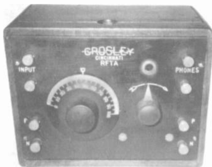
CROSLY MODEL RFTA – RFTA stands for "Radio Frequency Tuned Amplifier." This 1922 unit was designed to be used with the Harko Senior detector. (Ed Bell – Raleigh, NC)
