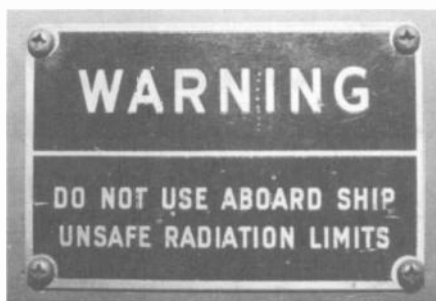
Figure 2. The red plate on the front of the Crosley REO warns against use aboard ship due to radiation from the radio's local oscillator.
