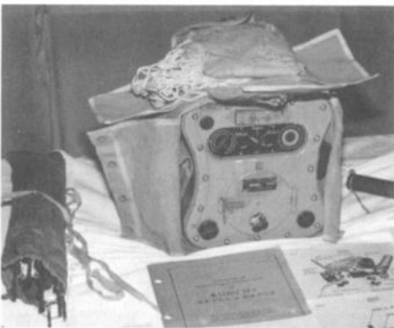
World War II, U.S. Navy transceiver, SCR 578-A. Emergency radio used in life boats and for downed pilots. Commonly known as the "Gibson Girl" radio.
