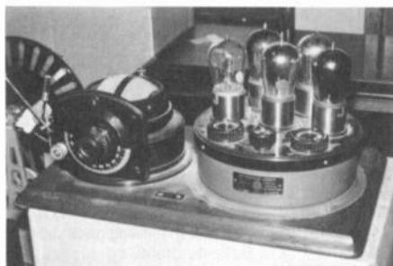
Four of the five Atwater Kent Model 5 breadboards at this year's meet. Clockwise from lower left: a flea market AK 5 that found its way into the auction; an early version Model 5 in the contest; a late version of the AK 5 in the contest, and another early version AK 5 contest entry. The early versions are noted by the name tag in the top, front center of the board.
