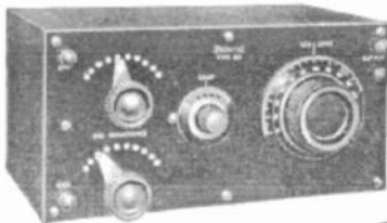
No. 60 Tuner (above), two tuned circuits for broadcast reception.
