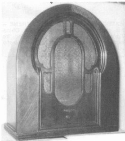
Figure 5. A Philco R-3 extension speaker with volume control. (Photo courtesy of Michael Prosisie.)
