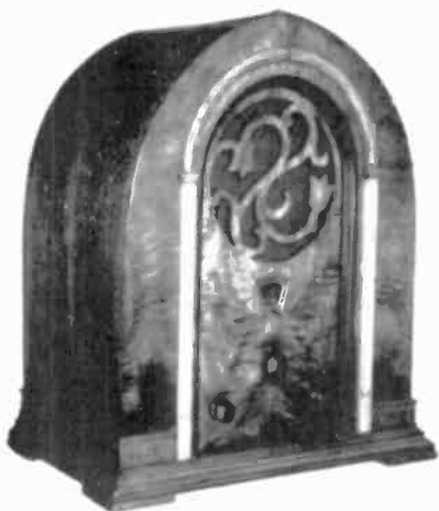
JACKSON-BELL MODEL 68 – This beautiful, 8-tube, 1931 cathedral, manufactured in Los Angeles, started my collection. It has a tulip cutout design in the speaker grille and a walnut cabinet. ( Andy King – Seattle, WA )
