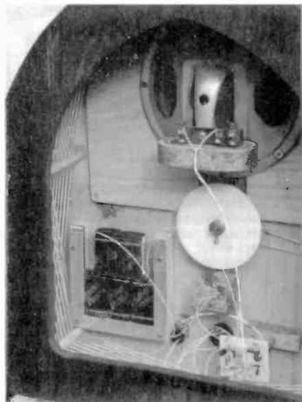
Figure 3. Rear views of the one-tube transistor cathedral radio showing the components used, including the built-in loop antenna.
