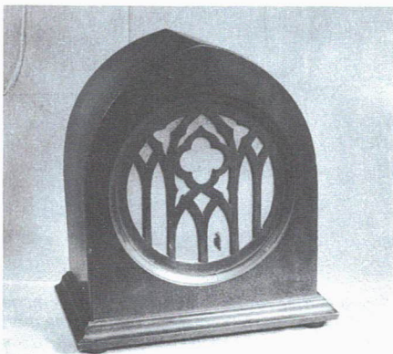
Figure 3. The Peerless Reproducer, a cathedral-shaped speaker popular in the late 1920s and still available in antique radio flea markets.
