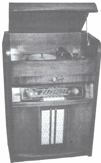
BRAUN FLOOR MODEL – This German floor model, circa 1950, has a 78 rpm record player beneath the curved front lid. Two swing-open doors below reveal storage space for records. The receiver has BC/SW/LW bands, a rotatable ferrite loop antenna, and a tuning indicator. It has 8 tubes, some of which are peanut tubes. (Randy King – Lincoln, NE)
