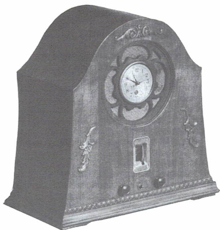
RADIO-CHRON CATHEDRAL – Although the model number of this ornate radio is unknown, the escutcheon and the thumb-wheel tuning capacitor drive are the same as those of the Gloritone Model 27, indicating that U.S. Radio and Television was the manufacturer. The tube layout is Type 80, 45, (3) 27s, and 24A. Help in finding the schematic for this radio would be appreciated. (Karl Stegman – Belleville, IL)
