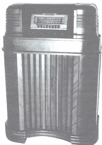
PHILCO MODEL 40-180 – Built in 1940, this 7-tube, 3-band, shortwave superhet has push buttons and frequency tuning ranges of 540 to 1550 Kc, 1.5 to 3.4 Kc, and 6.0 to 18 Mc. ( Albert D'Ambra – Rocky Point, NY )
