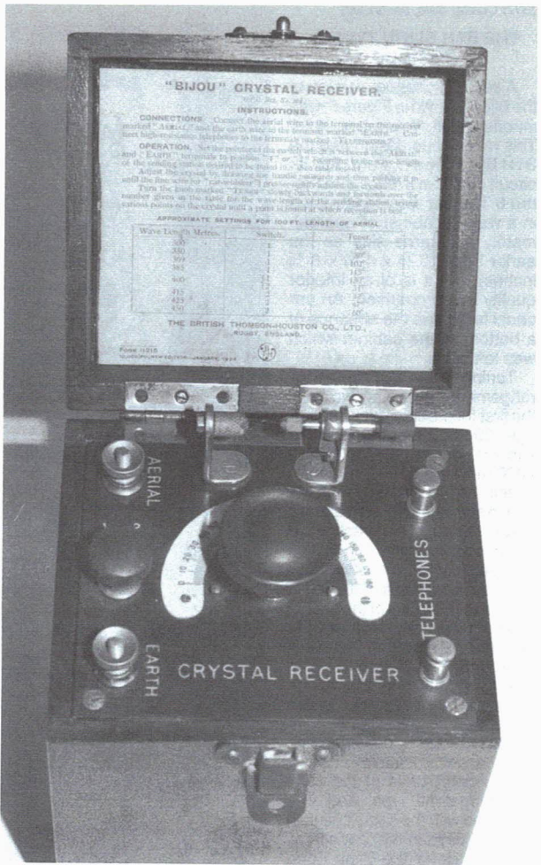
Figure 3. The BTH Bijou Type C, Form B crystal set with crystal detector in the rear.
