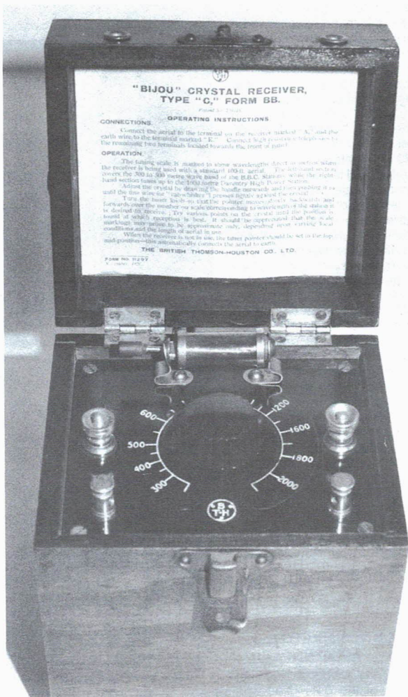
Figure 5. The BTH Bijou Type C, Form BB crystal set.
