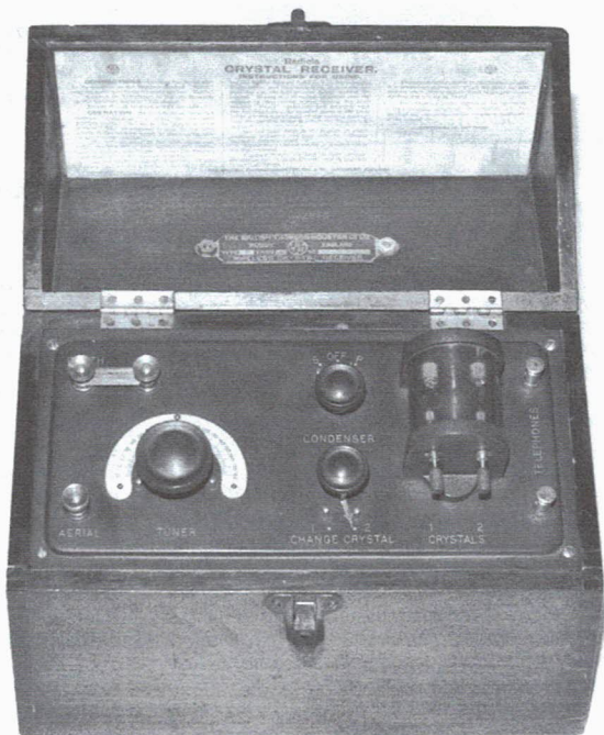
Figure 1. The BTH Model A crystal set with twin detectors on the right.
