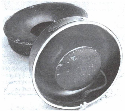
Figure 5. Bottom view of the Kodol base showing the Utah driver unit.
