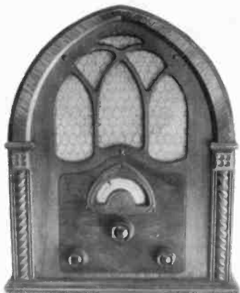
ATWATER KENT 82Q - Manufactured in 1931, this battery-operated version of the Model 82 cathedral radio has seven tubes and was one of AK's first superheterodyne radios. Tuning, volume, and tone controls are in front; a local-distance switch is mounted on the left side of the cabinet, while the on-off switch is on the right side. (Ron Ramirez - Providence, KY)
