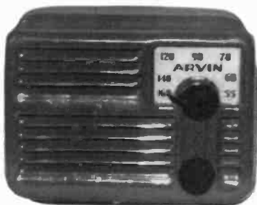
ARVIN MODEL 444 - This (1947?) red Arvin, metal radio, (Chassis Re-200) has a tube line-up of 12SA7, 12SQ7, 50L6GT, and 35Z5. At 6.5 x 5 x 4 inches, this radio is near the lower limit in size for any radio with four octal tubes. (David Kraeuter - Washington, PA)
