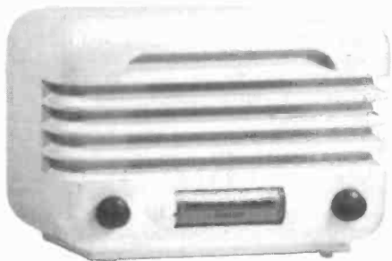
AIRLINE 93BR-421B - A compact superhet in a streamlined, white, plastic cabinet, this model has a slide rule dial that is unusual in a very low priced set. ( Fred Geer - Jacksonville, FL )
