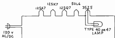
Figure 3. Panel lamp connection to tapped rectifier tube heater.
