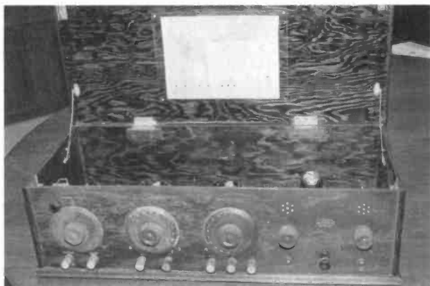
Figure 3. Neurodyne built with Fada components, possibly an engineering prototype.
