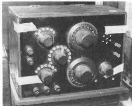
One-tube receiver, quite possibly a factory set, but no identification. A well-built radio.
