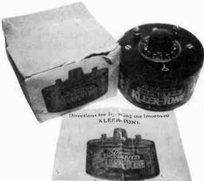
RESEARCH LABORATORIES, INC. KLEER-TONE - Produced in the early 1930s, this unit appears to be a type of wave trap advertised as easy to connect and adjust and sure to make a general improvement in radio reception on any type of set. (Steve Carter - Plainfield, IN)
