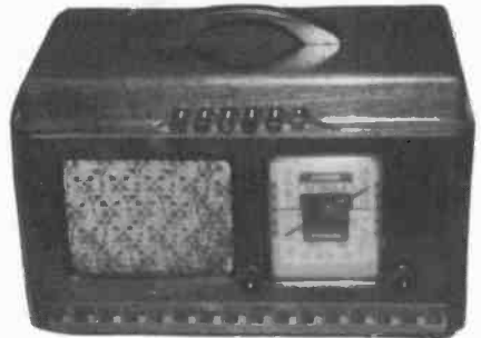
DETROLA MODEL 310 - This late 1930s cabinet features a carrying handle and beautiful inlay work across the bottom front consisting of ninety-nine pieces. The set uses seven octal tubes and has six electronic push buttons. It has an early, built-in loop antenna, and operates on AM/SW. (Victor G. Marett - Miami, FL)
