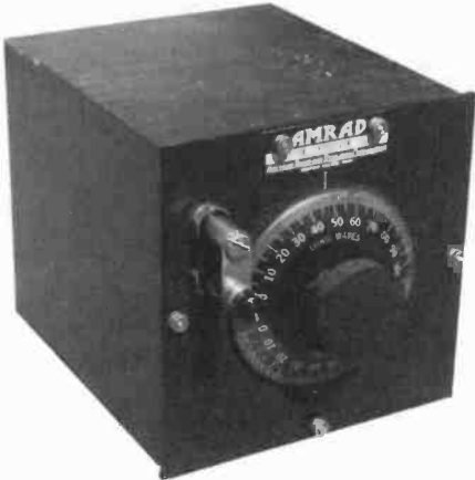
AMRAD CRYSTAL RECEIVER - This is the Type 2575 crystal set with a unique plug-in detector unit. It was manufactured by the American Radio and Research Corporation of Medford Hillside, Massachusetts, and sold in 1922. (Dave Crocker - Duxbury, MA)
