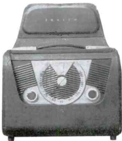
1950 PORTABLE - Zenith produced this Model H503 with a chassis number 5G41. It is covered in black leatherette with a gold-tone dial, red numbers and copper knobs surrounded by plastic. It runs on battery or 110 volts AC. (Steve Hartwich - Kansas City, MO)
