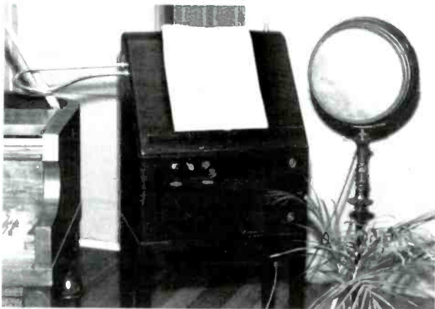
Figure 1. The RCA Model AR-1264 Theremin. Although it is shown here with an RCA Type 100 drum speaker on an ornate stand, the RCA Victor Service Notes for 1929-1930 recommends using the RCA Type 106 console speaker with the tapestry front.
