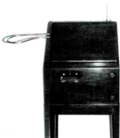
Figure 2. The Theremin control unit showing the vertical pitch and horizontal volume control rods. On the front are the few dials for adjusting the electronics and the on/off switches.
