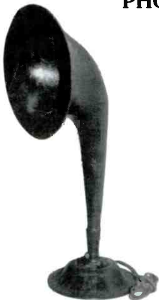
BRISTOL BABY AUDIPHONE - This 23" high horn with a 10-1/4" bell was manufactured by the Bristol Company of Waterbury, Ct., in 1924. The base is metal, and the horn is of fiber material. (Walter Worth - Wollaston, MA)
