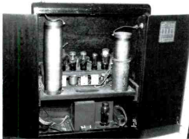
Figure 3. The rear view of the RCA Model AR-1264 Theremin showing the electrical power unit chassis and tubes.
