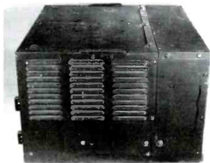
Figure 2. The RAO-2 receiver showing the bolt-on sheet metal extension to add three inches to the rear of the set.
