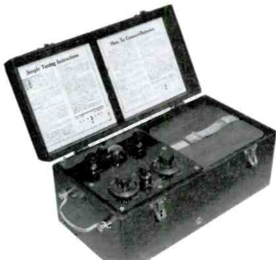
1922 KENNEDY PORTABLE - The Colin B. Kennedy Type 311 one-tube portable receiver is a self-contained unit with space for batteries (or amplifier) in the compartment to the right of the panel. A wooden plate fits over the battery area with a strap to hold a pair of Kennedy headphones when the cover is closed. (Dave Crocker - Duxbury, MA)
