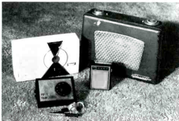
Figure 1. Early transistor radios. Back view: Philco Model T-7, Raytheon Model 8-TP. Front row: Model PP-7 transistor kit radio, Sony Model TR-730.
