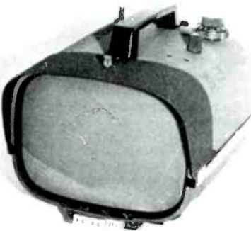
Figure 4. Sony's first transistor TV, the Model 8-301W, circa 1961.
