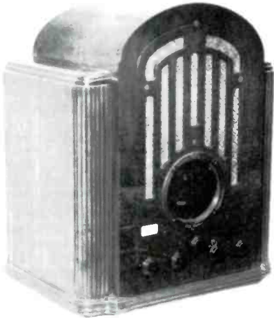
RCA MODEL 128 CATHEDRAL - The only repair needed on this 1933 set was that two pieces of veneer had to be replaced; otherwise it ran beautifully. This seems to be the norm for these early sets. It works with AC voltage, and is a six-tube, with three bands. ( Walter Worth - Wollaston, MA. )
