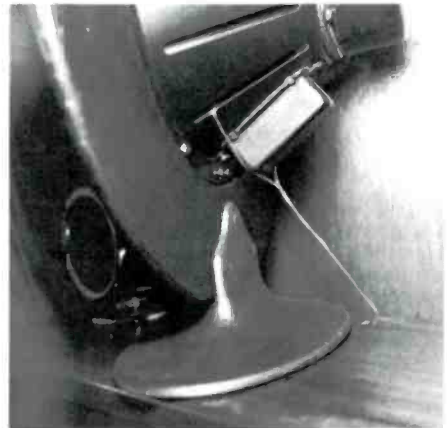
Figure 5. Wire and hook anchor used to secure the Rola speaker.
